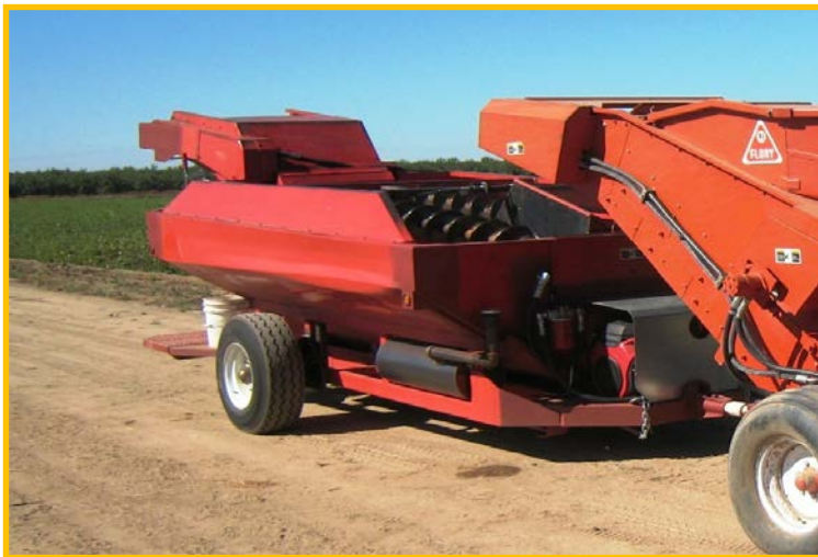
Self contained hydraulic system for operating augers, autosampler and elevator
