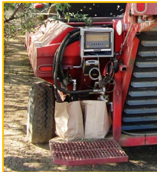
Trimble GPS acts as datalogger to collect continuous yield data
