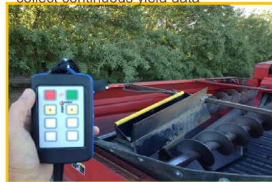
Wireless controller for hydraulically operated auto sampler
