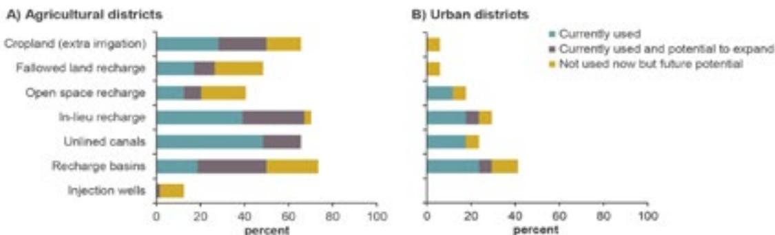
PPIC. Ag Water Districts see significant potential for expansion in the recharge methods covered in this guide.
