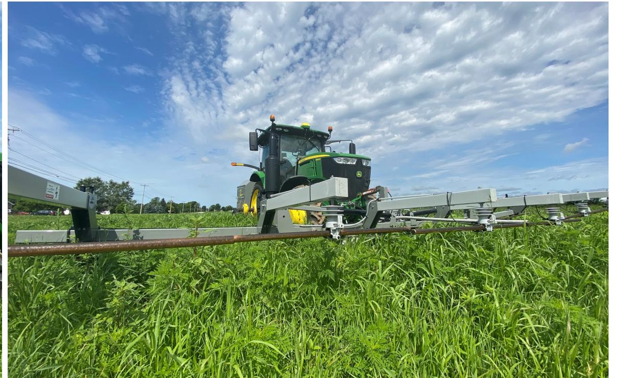
WEED ZAPPER™ IS A TRACTOR-TOWED, PTO-DRIVEN GENERATOR THAT PRODUCES 100,000+ WATTS OF ELECTRICITY
